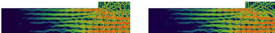
Figure 2.7: Absolute square of the electron (left, |u|^2 ) and hole (right, |v|^2 ) wavefunctions calculated for a quadratic Andreev billiard ( linear dimension D = 1 , attached to a lead with width W = 0.8 ). k_F = n_y * \pi / W = 21.5 * \pi / 0.8 , where [n_y] is the number of open modes in the lead. Shown are false color plots, black areas represent zero amplitude, red the highest. The state shown has an excitation energy of \varepsilon = 0.558\Delta
