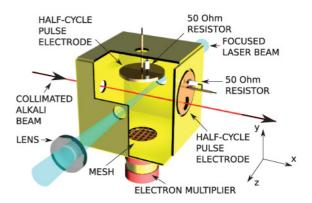
FIG. 1. (Color online) Schematic diagram of the apparatus.
